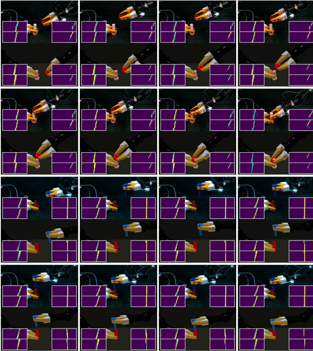
Figure 10: Qualitative tactile signal alignment. Side-by-side real-to-sim replay trajectories for Assembly #1 and #2. Each pair shows synchronized real and simulated frames with tactile maps, highlighting matched contact location and evolution.
